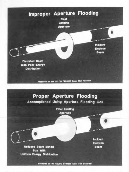
the electron gun structure). Since these stray electrons are not controlled by the G1-cathode bias, even when the CRT beam is cut off, such electrons will continue to reach the phosphor screen and expose the film when no exposure is called for.
