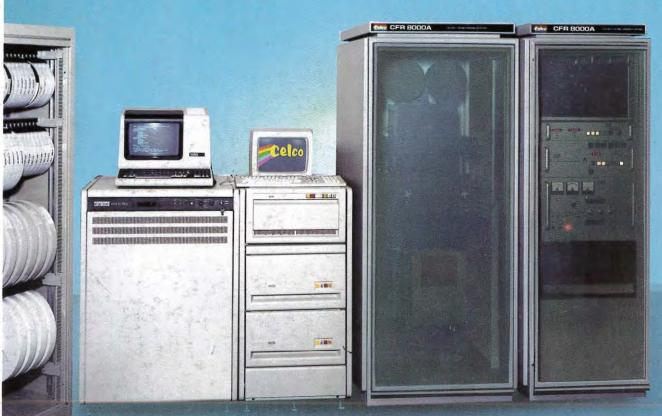
CELCO CFR 8000A Color Film Recording System shown above with DEC-VAX option.
