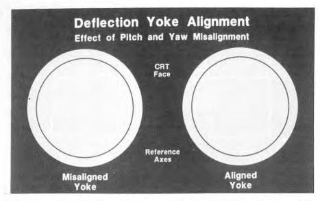
with an accurate grid pattern projected on the CRT face, and adjustment made to achieve the best balance of symmetries around the edges.
